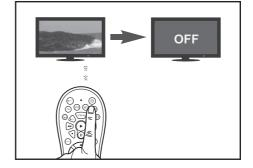
4 When the device is off, immediately press and release **OK** to save the code. The blue LED indicator will turn off.
