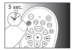
Point at your device with the universal remote. Then press and release **ψ** to start searching the code for your brand. A different infrared signal is sent every 2 seconds as the universal remote searches, indicated by a blue flash.
